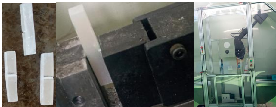
Figure 5 Charpy Izoid Impact testing machine setup
