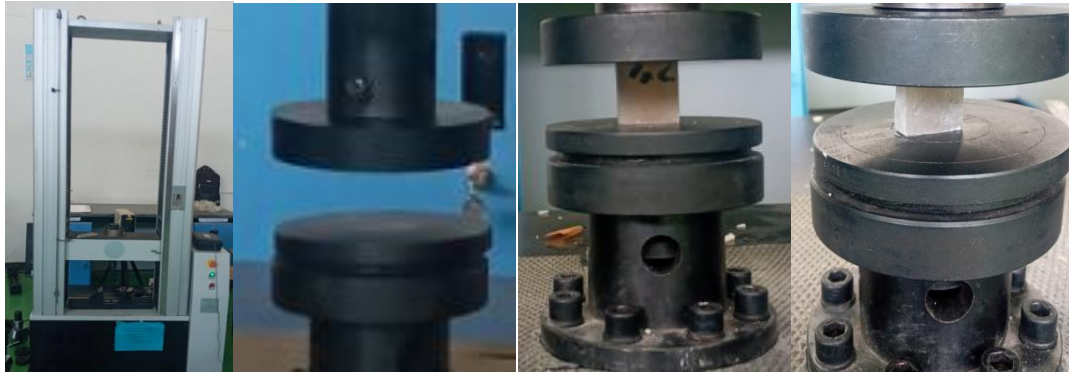
Figure 6 Compression testing machine setup
