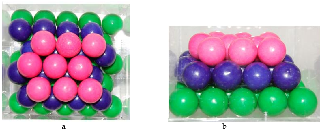
Figure 4. Cubic close-packing model. a) top view of ABCABC... layer, b) side view of ABCABC... layer
