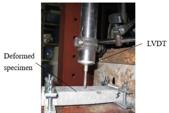
Figure 4 Measuring deflection using LVDT
