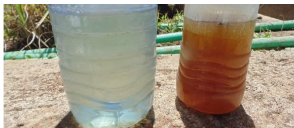
Figure 2: Colour change in the wastewater after (left) and before (right) treated with the constructed wetland
