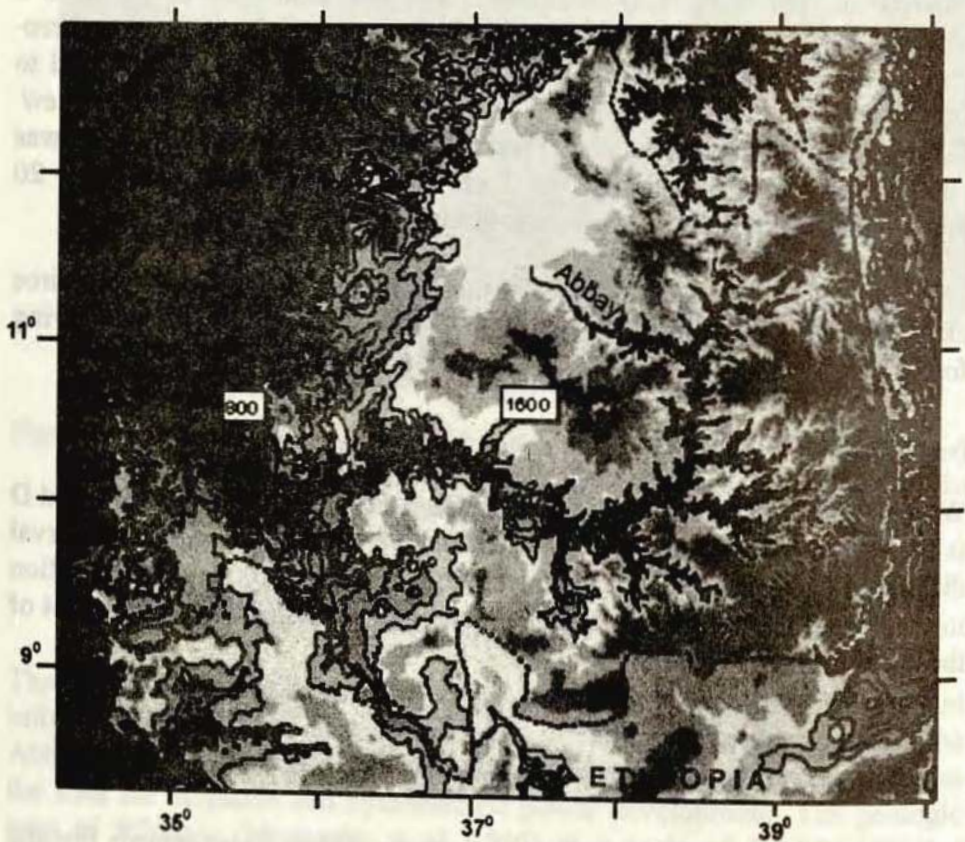
Figure 2: Topographic map of the Blue Nile Basin created from DEM using Arc View GIS software.
